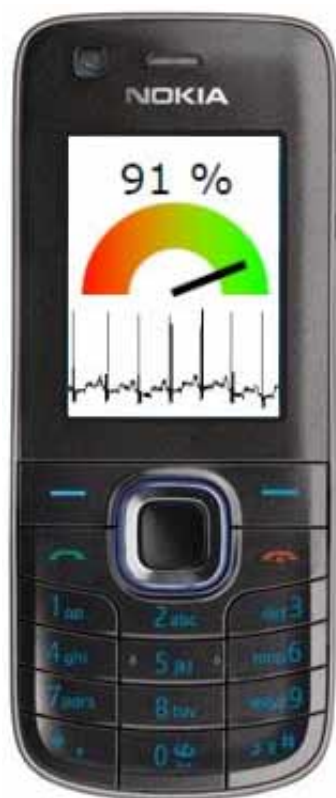
Fig. 4 Picture of NFC enabled mobile phone Nokia 6212 classic running the HF APP. Its screen shows the ECG signal streamed by the sensing device and the calculated signal quality level.
