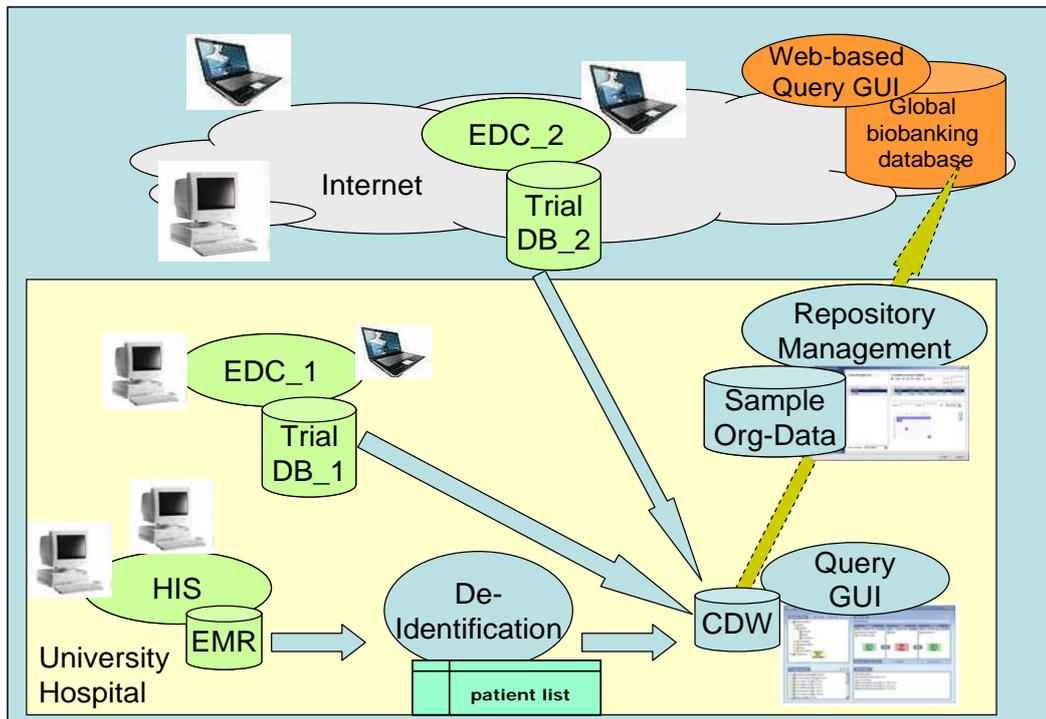
**Fig. 1** Architecture and core components of a biobanking IT infrastructure: primary data sources in green (EDC = electronic data capture system, DB = database, HIS = hospital information system, EMR = electronic medical record); biobanking core components in blue (Org-Data = organizational data on samples and storage locations, CDW = clinical data warehouse, GUI = graphical user interface); integration with transnational, European or world-wide biobanking networks in orange.
