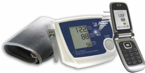
Figure 1 Blood pressure meter UA-767 Plus NFC (AND, Japan) with integrated NFC module (AIT Austrian Institute of Technology, Austria) to allow for wireless transmission of measurement values based on the ISO 14443 standard.
