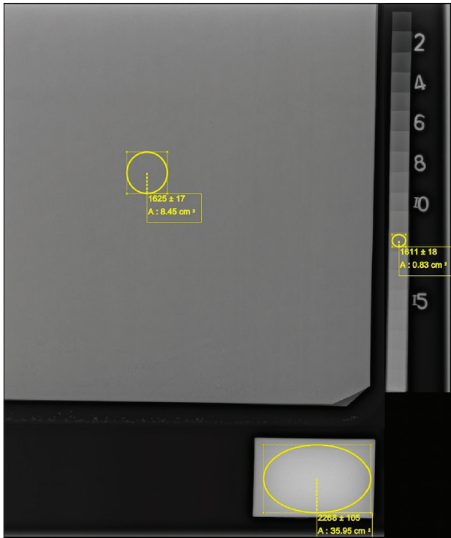
Figure 4: Regions of interest showing pixel intensities of apron, step wedge, and lead block from digital radiographic images
