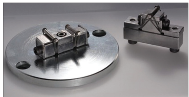
Figure 3: Flexural test device. Superior and inferior support view
