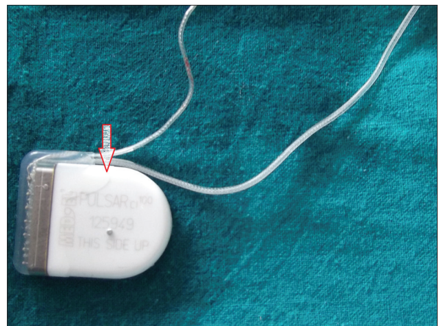
Figure 9: Fracture line on the receiver stimulator
