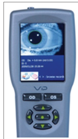
Figure 5: Pupillometer and its measure
