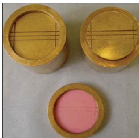
Figure 1: Stainless steel test die constructed according to American dental association specification no: 18 for alginate impression material
