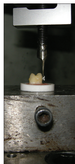
Figure 1: Position of the tooth and bracket in the Zwick testing machine, prior to the debonding process
