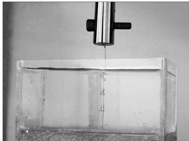
Figure 2: Device used in frictional force test
