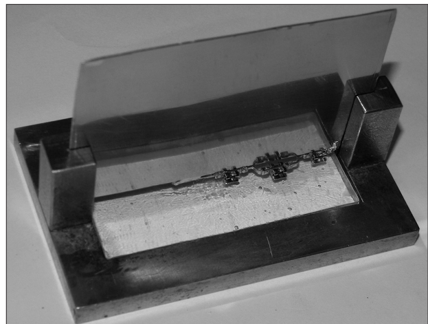
Figure 1: Device used to standardize the bonding procedure
