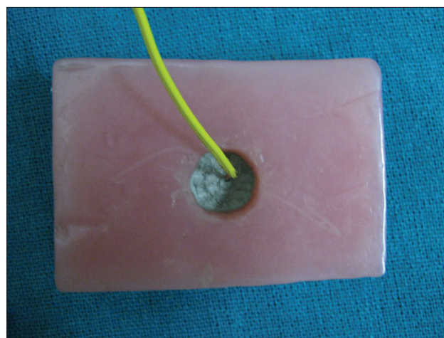
Figure 1: Amalgam with thermocouple inserted in hollow pulp chamber
