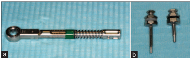
Figure 21: (a) Adjustable mechanical torque wrench (b) Mechanical screw-driver: Various lengths
