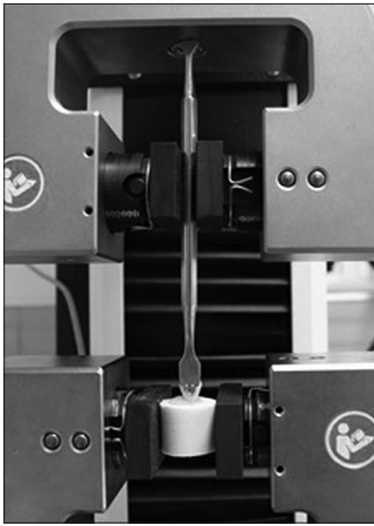
Figure 1: Setup for bracket debonding
