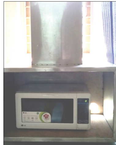
Figure 1: Microwave oven placed in a stainless steel enclosure fitted with vent opening to the exterior environment
