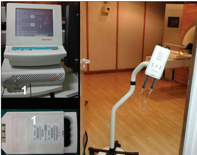
Figure 6: MR pressure injectors (Medrad Spectris). Functional issues include (A) battery operations (12 V DC, 25 A) which charges at console, discharges at MRI suite (B) non-ferromagnetic status and (C) availability of vendor specific sensors such as keep vein open for intermittent injection
