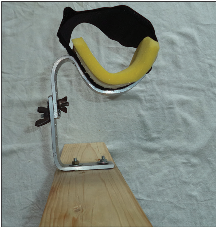
Figure 2: The height and angle of the foam lined arm support can be adjusted with the help of the metallic components with holes
