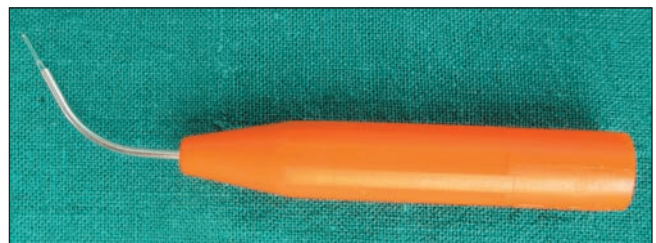
Figure 6: A fiber-optic wire tip of 200 \mu m
