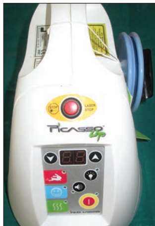
Figure 5: Diode laser unit (810 nm)
