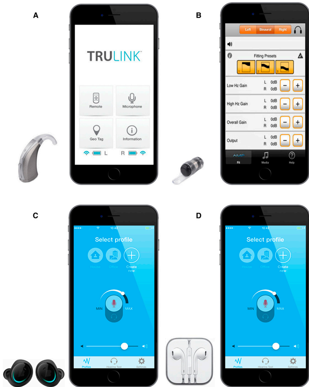
Figure 2. Images of the smartphone-connected listening devices trialed in the study. (A) Smartphone-connected hearing aids: behind-the-ear Starkey Halo i110 hearing aids, adjusted via the TruLink app. (B) Personal sound application product: in-the-ear Starkey AMP Personal Amplifiers, programmed and adjusted using dual-tone multifrequency signals via the accompanying AMP app. (C) Smartphone “hearing aid” app with wireless hearable: the Petralex smartphone app used with Bragi Dash wireless earphones that pair with the user’s smartphone via Bluetooth. (D) Smartphone “hearing aid” app with wired earphones: the Petralex smartphone app used with standard wired earphones provided with the user’s smartphone. (This figure appears in color in the online version of this article.)
