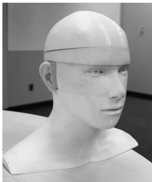
Figure 1. Image of the new probe-tube placement training simulator with a 3D-printed head and silicone ear model. The camera system is mounted inside the head to give the user real-time feedback on the placement of the probe inside the ear canal.
