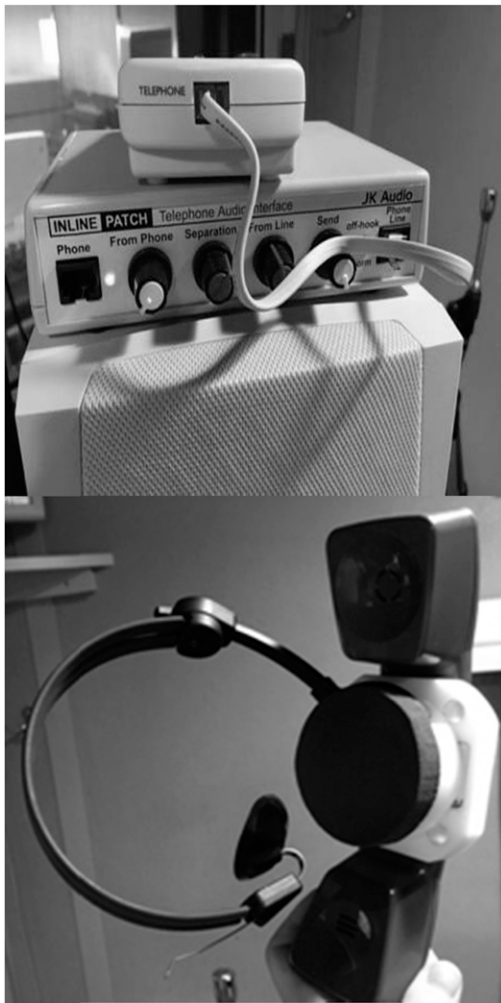
Figure 2. Equipment used to preserve calibration of speech stimuli from the audio CD player to the telephone handset (top panel). Telephone handset affixed to a custom-manufactured moveable headband providing consistent placement during testing of speech recognition (bottom panel). Ledda, Kimberly. "Custom-made headband." 2016. Digital File Type.
