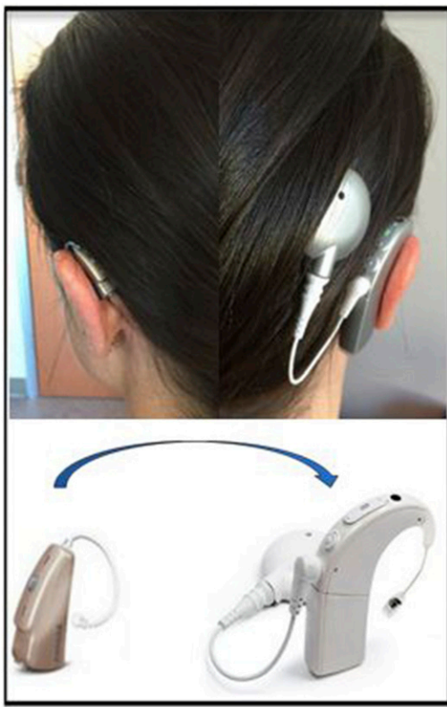
Figure 1. Customized initial CROS prototype from Advanced Bionics designed to wirelessly route the acoustic signal from the non-implanted ear to a Naida CI processor.
