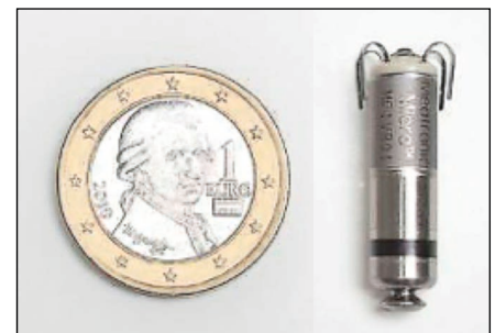
Fig. 4 The Medtronic Micra TPS leadless wireless pacemaker
