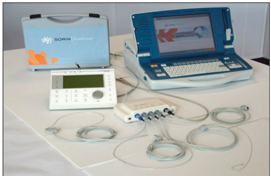
Fig. 6 The SonRmap platform, designed by Sorin, to assist the implantation of the device based on the microaccelerometer sensor
