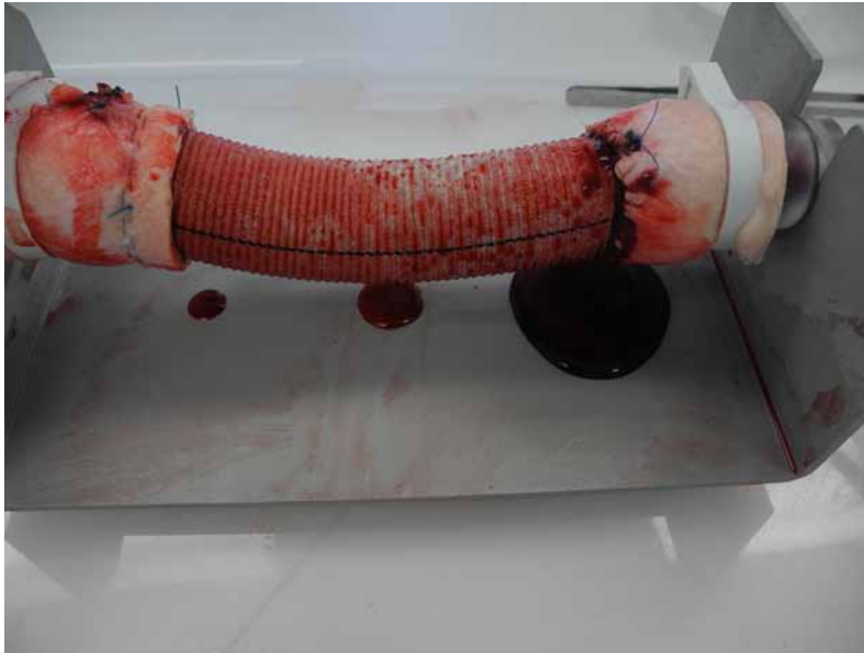
Figure 7. A picture from one of the first experiments is shown. A Dacron tube graft is interposed between two ends of a bovine aorta, the left side stapled with the device described in this report and the right side hand-sewn. The aorta-graft is then filled with bovine blood with a syringe loaded onto a pump, and the pressure is gradually increased. The pressure was <30 mm Hg when this picture was taken, and there was already a pool of leaked blood on the hand-sewn side.
