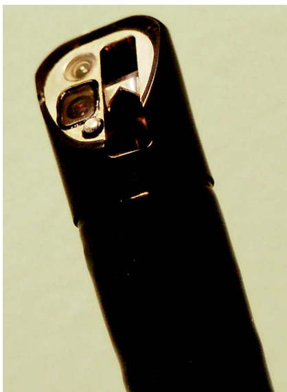
Fig. 3 Prototype upper scope with an oblique-viewing angle.
