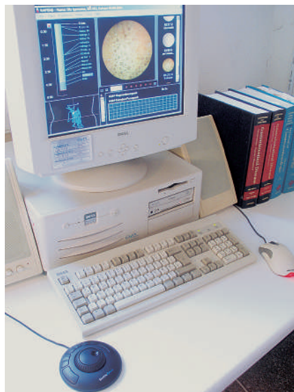
Figure 2 Placing the jog/shuttle control on the left and the mouse on the right side appeared to be the most practical solution.
