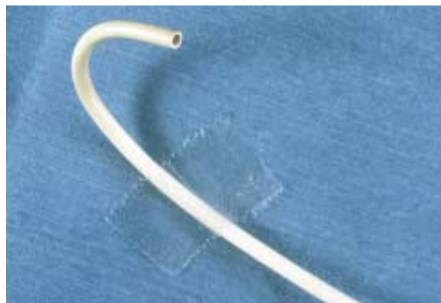
Figure 2 The cut end of the extracted tube was not sharp and no apparent deformation was seen
