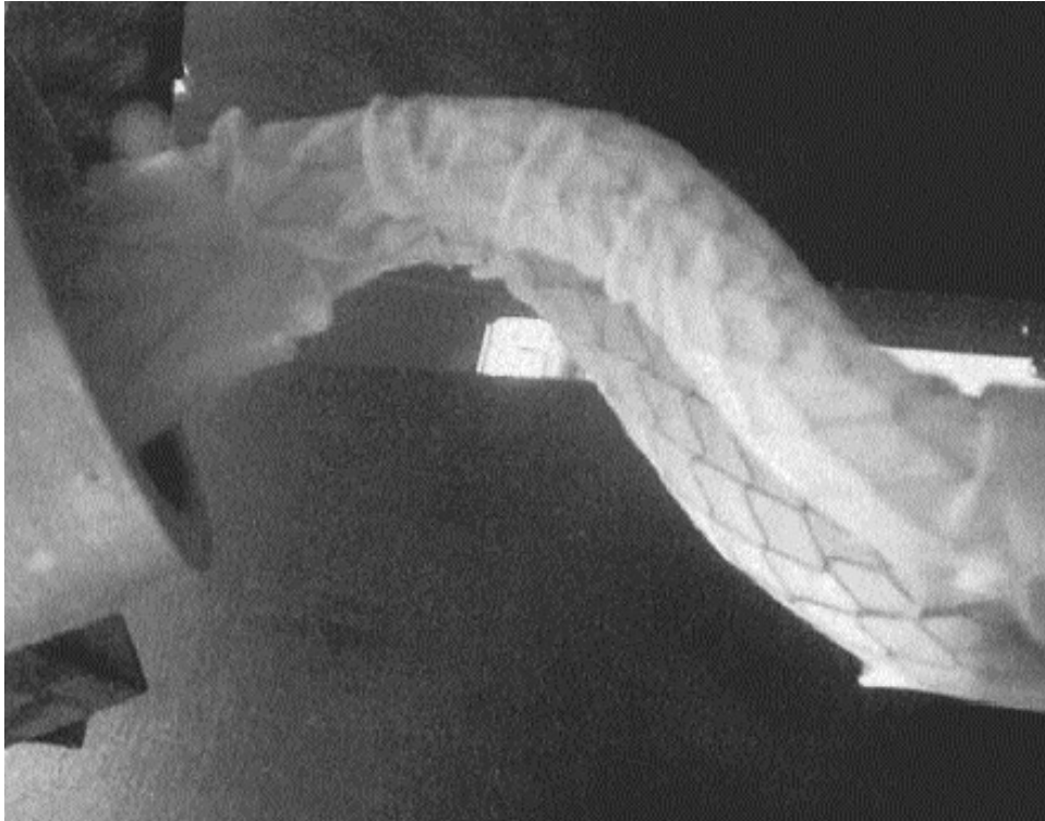
Fig. 6 This shows a Vanguard stent graft in an apparatus simulating the angulation of implanted iliac limbs. The effects of pulsatile forces can be studied by ex-vivo testing. (From: Beebe HG. Late risks of endograft for aortic aneurysm: observations from the United States Vanguard trial. In: Greenhalgh RM, ed. The Durability of Vascular and Endovascular Surgery . London: W.B. Saunders Co. Ltd; 1999, p. 415, with permission.)
