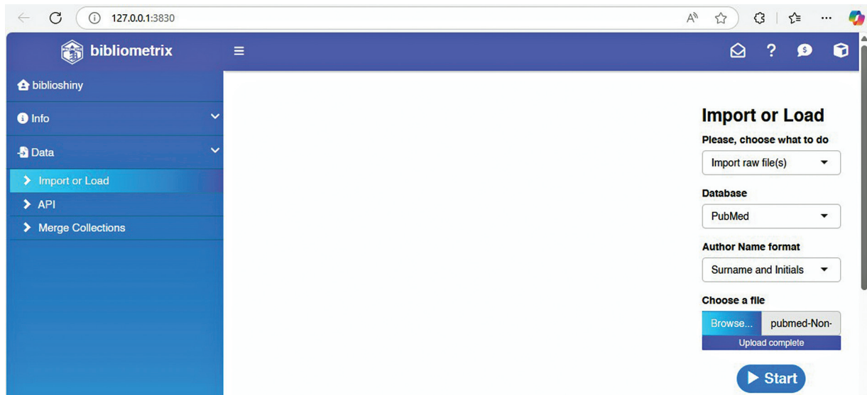
Fig. 3 A screenshot of Biblioshiny where data import button (Import or Load) is showing on the left side and import options (file types, database, author name format) are showing on the right side of the image.
