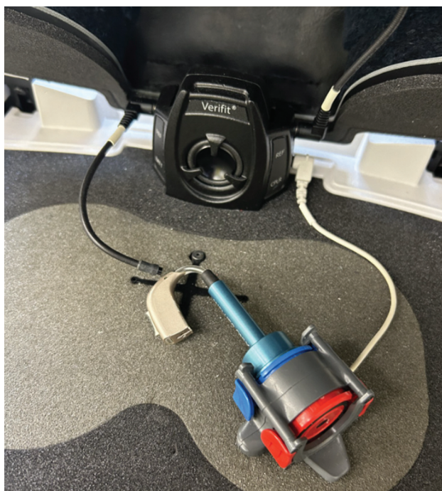
Figure 6 Attaching a behind-the-ear to an HA-2 coupler.
