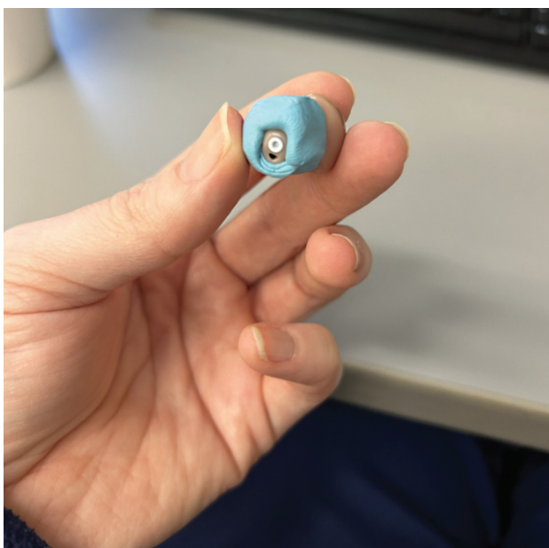
Figure 8 Using putty to create a seal between the hearing aid and the coupler.
