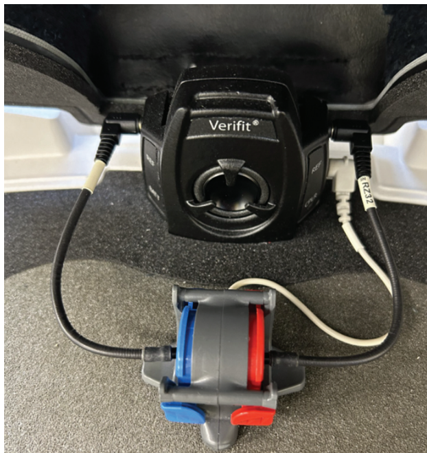
Figure 2 Test box leveling setup. Note that the two reference microphones are as close as possible to the coupler microphones.
