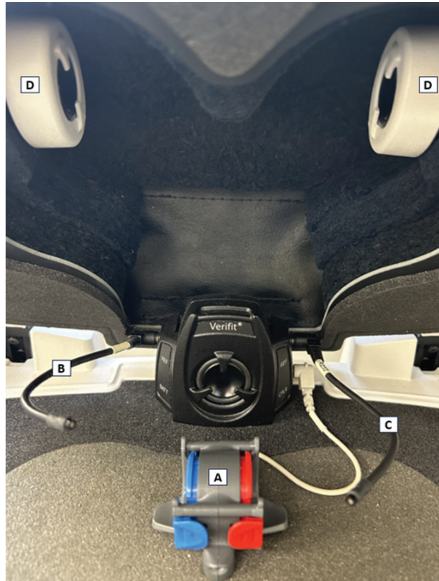
Figure 1 Parts of the test box. (A) Binaural coupler microphone; (B) reference microphone (left); (C) reference microphone (right); (D) speakers.
