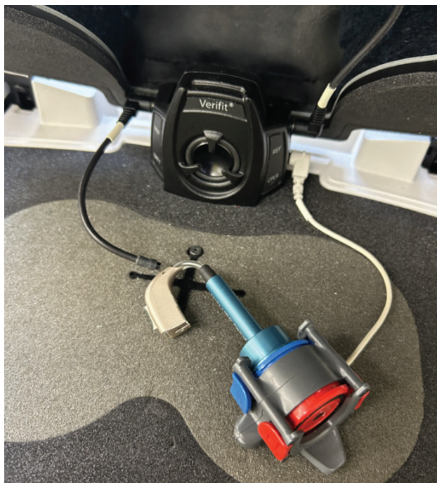
Figure 6 Attaching a behind-the-ear to an HA-2 coupler.
