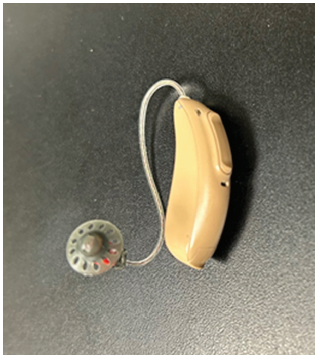
Figure 7 Receiver-in-canal with open dome.
