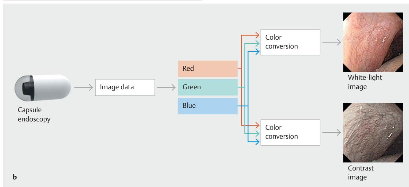
► **Fig. 1** **a** The capsule endoscope was equipped with selected white light-emitting diodes, which provided increased illumination intensity in the blue light spectrum (the main absorption range of hemoglobin). **b** Contrast capsule endoscopy system configured predominantly with blue light and green light using the color illumination system.
