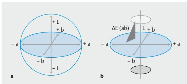
► **Fig. 2** **a** Lab color space as defined by the International Commission on Illumination (CIE). **b** Color difference ( $\Delta E$ ) was calculated using the following equation:  $\Delta E = (\Delta L^2 + \Delta a^2 + \Delta b^2)^{1/2}$  where L represents lightness, a the red-green component and b the yellow-blue component.
