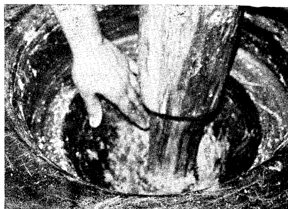
Fig. 6. The mechanism of hand injury by an oil extracting Kolhu machine.
