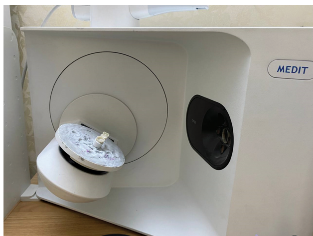
Fig. 2 Scanning of the inner surface of each abutment.
