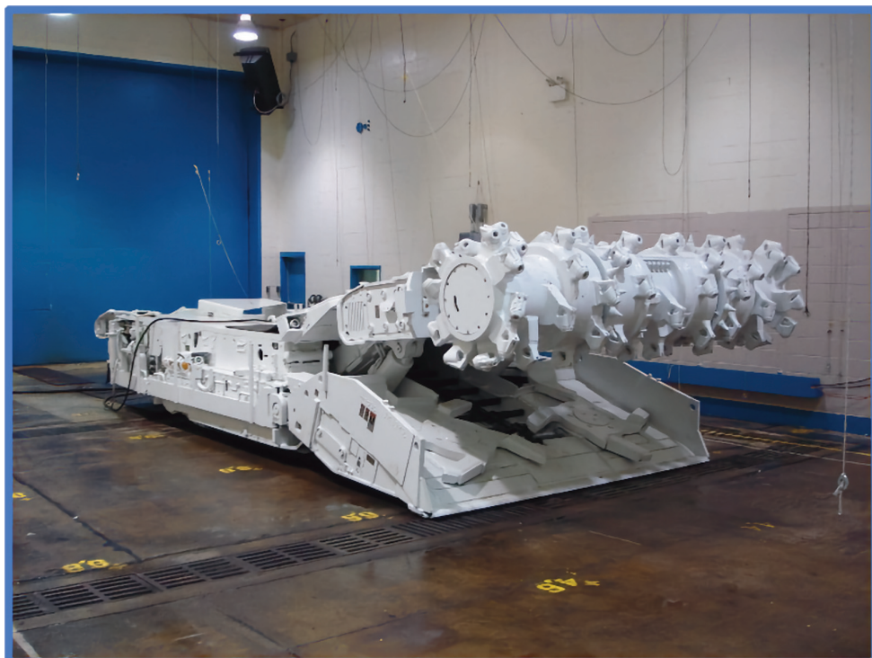
Figure 9 Continuous mining machine prior to sound power testing in the ATC.
