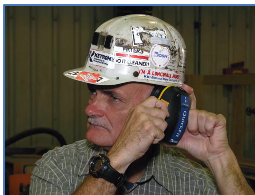
Figure 20 The QuickFit is a simple method to test ear plug insertion effectiveness.
