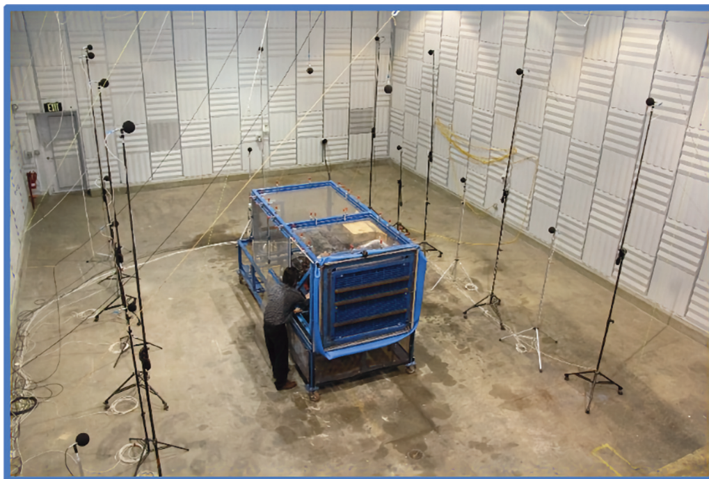
Figure 3 Hemi-anechoic chamber set up for sound power testing per ISO 3745.
