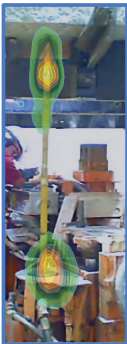
Figure 15 Beamforming analysis confirms that the drill steel is a significant noise source on a roof bolting machine.
