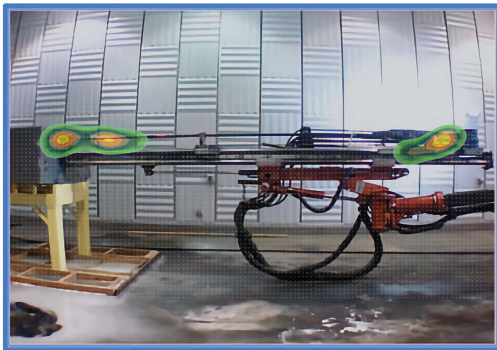
Figure 7 Beamforming analysis locates two noise sources on a jumbo drill.
