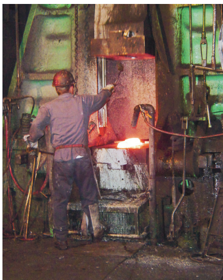
Figure 1 Hammer operator at a pneumatic forge hammer. (Photo by NIOSH.)
