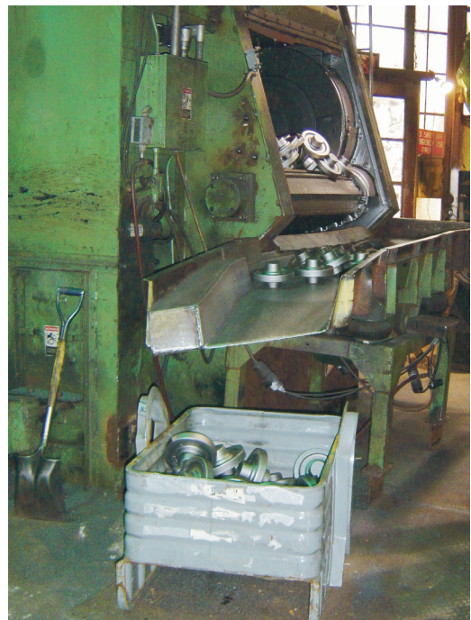
Figure 7 Forgings being dumped from a shot blast onto a vibrating conveyor pan and moving down the conveyor to fall into a metal bin. (Photo by NIOSH.)
