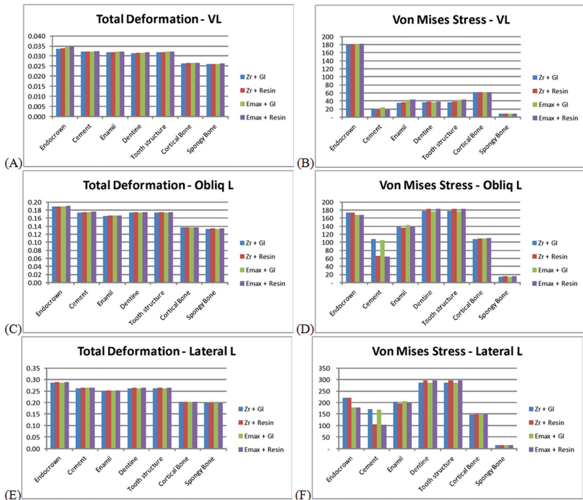
Fig. 3 Comparison of different materials stresses under different angles loading. Vertical loading (A) total deformation, (B) Von Mises stress; oblique loading (C) total deformation, (D) Von Mises stress; and lateral loading (E) total deformation, (F) Von Mises stress.
