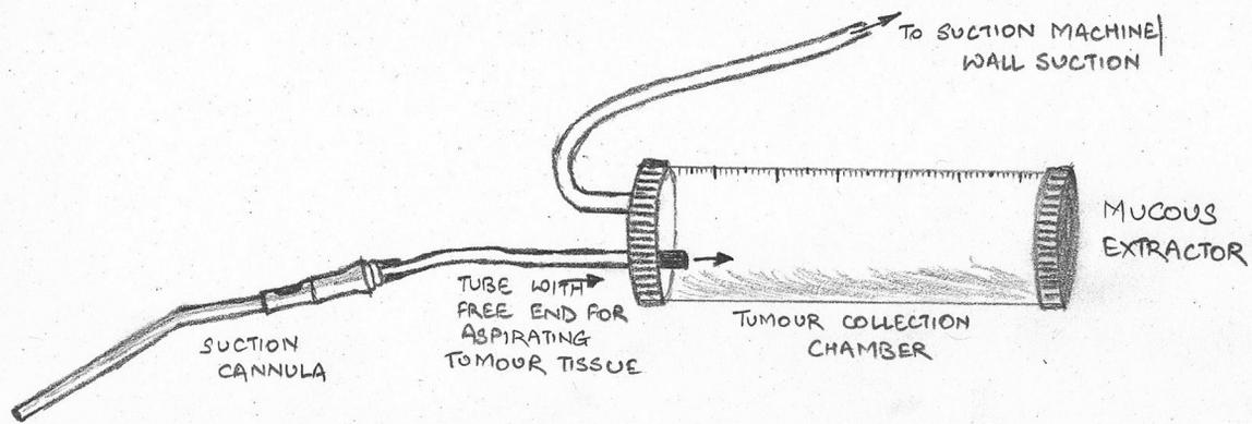
**Fig. 1** Hand-drawn diagram showing the various parts of the mucous extractor device and its application for suction biopsy.
