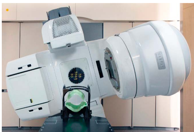
► Fig. 1 Modern linear accelerator with assembly for mask and stereotactic head frame.
