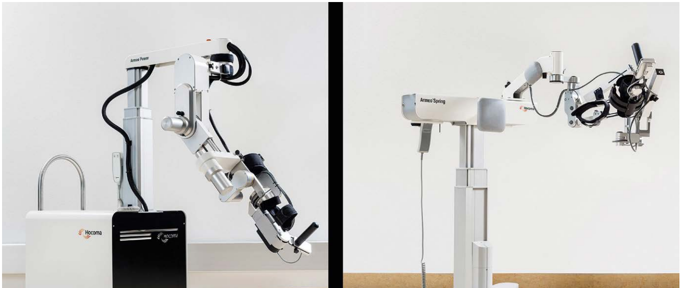
► Fig. 2 ArmeoPower and ArmeoSpring. The ArmeoPower system (Hocoma, left) uses pneumatic drives to perform movements of the upper extremity, including the shoulder (exoskeleton). In comparison, the ArmeoSpring system (Hocoma, right) is a resistance system requiring activity of the rehabilitant's affected limb. Guidance of the movement is provided in the distal region; in contrast, the shoulder does not receive proximal guidance but is included in the chain of movements.
