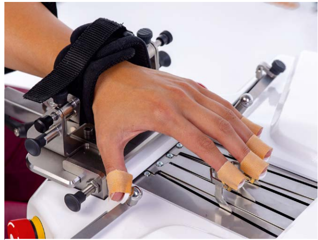
► Fig. 1 Amadeo. This device is an end-effector using an electric drive that via fixation of the wrist supports the position and force of each finger, including the thumb.
