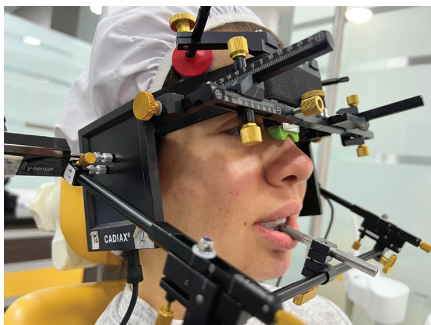
Fig. 1 Photo of double electronic stylus in place, against the flag, kept in constant contact by magnetic tips, ready to measure the translation, rotation, and transversal components of the movement in each joint.
