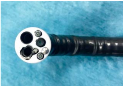
Fig. 2 The two-channel forward-viewing endoscope with an outer diameter of 1.8 mm, a field of view of 120°, a working length of 1030 mm, and two large forceps channels of 2.8 mm and 3.7 mm, the former having a forceps elevator.
