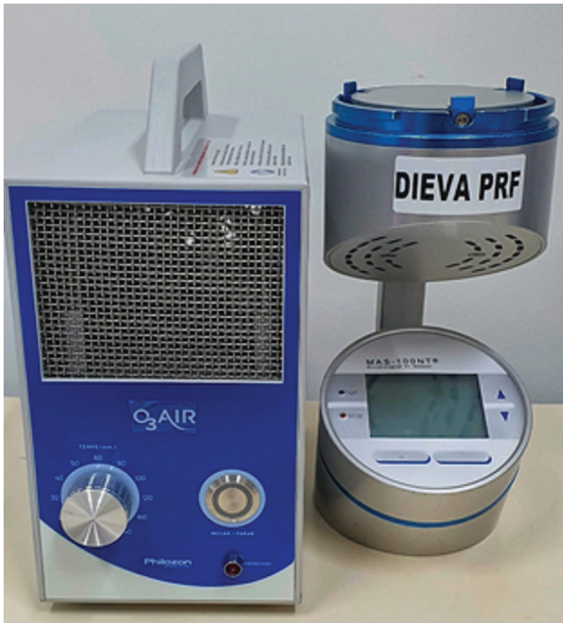
Fig. 1 The O 3 air ozone generator and microbial air monitoring system (MAS-100).
