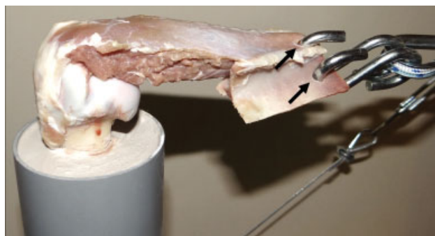
Fig. 2 Scapular foramina for the fixation of the infraspinatus muscle (anterior view). Two perforations were made 1 cm from the medial edge of the scapula, separated by 1 cm on each side of the scapular spine, with a 5.0-mm drill bit, to hook the osteotomized fragment to the load cell (anterior view).
