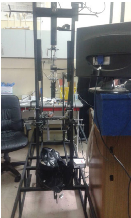
Fig. 2 The model consisted of three fundamental parts: a modular support with adjustable height, an adjustable support for guidance of the suture system, and a linear actuator with an intermediate load cell. The humeral shaft was fixated with a metal clamp.
