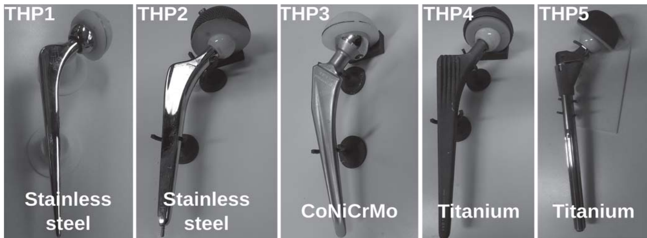
Fig. 1 Head and stem pictures of the five implants used in the present study. Prostheses were placed on plastic stands in order to be above the bottom of the container and surrounded by gel.
