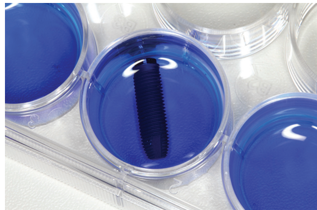
Fig. 3 Dental implant immersed in toluidine blue O (TBO) (100 µg/mL) for 1 minute before irradiation.
