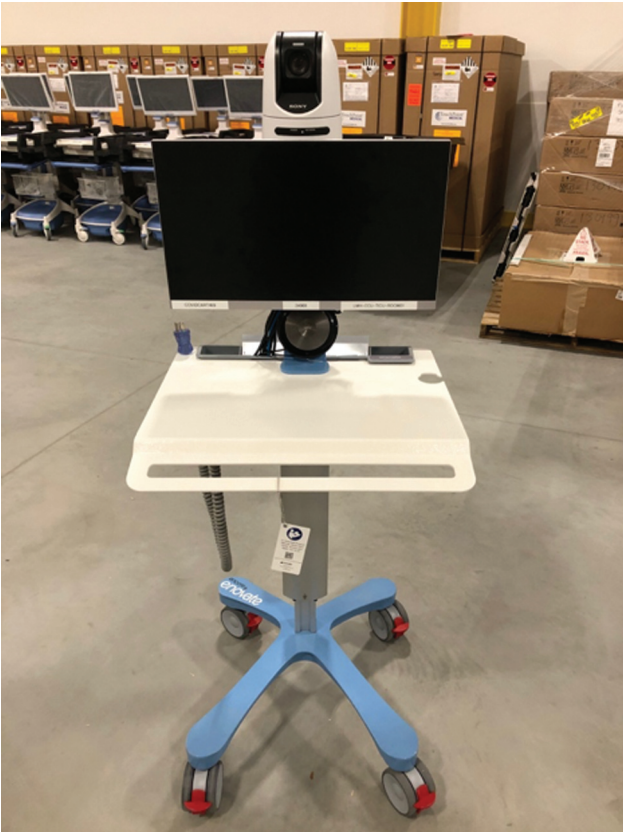
Fig. 2 Example cart built for intensive care units with high-resolution pan, tilt, and zoom camera.
