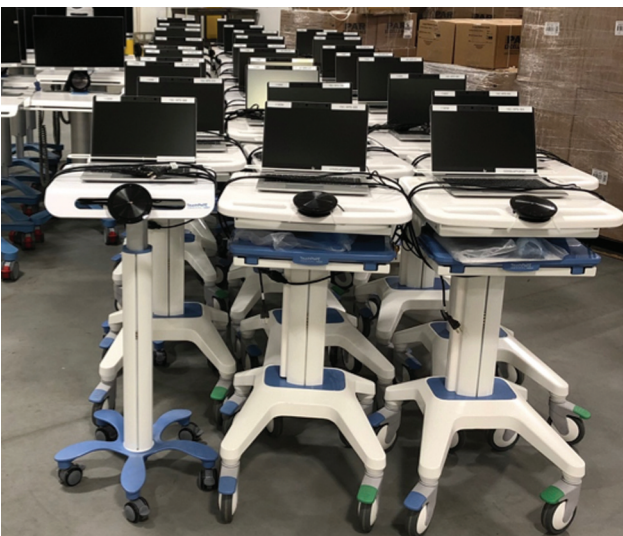
Fig. 3 Laptops on carts with external speaker and microphone for higher audio quality.
