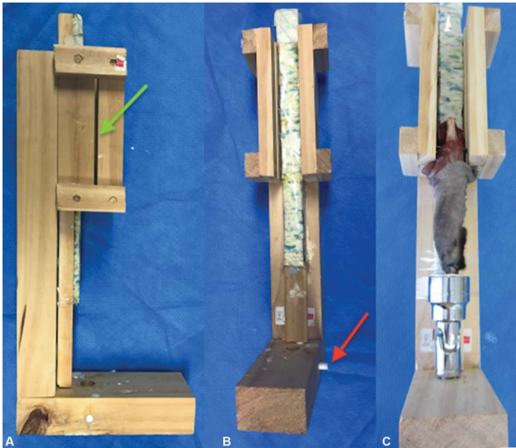
Fig. 1 Part A shows side on view of testing jig, B shows frontal view of testing jig without a mounted specimen and C shows frontal view of testing jig with a mounted specimen. The jig was constructed from wooden blocks. The specimen was suspended from a carbon rod with sliding insertion between parallel blocks to allow for adjustment of the limb position according to limb length. The wooden dowels in the base of the jig were secured centrally to fix the extension drive in a pronated or supinated position using a clamp. The green arrow points to the gap between parallel blocks that allowed for sliding insertion of a carbon rod, with the height adjusted to limb length. The red arrow highlights wooden dowels that are secured centrally within holes to fix the extension drive in a pronated or supinated position between computed tomography scans.
