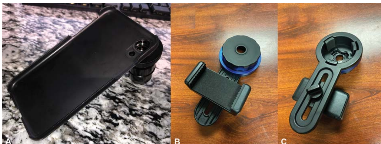
Fig. 1 Two different slit lamp adapters (A, for iPhone 10) and a universal slit lamp adapter demonstrating adjustable smartphone holder (B) and eyepiece adapter (C).
