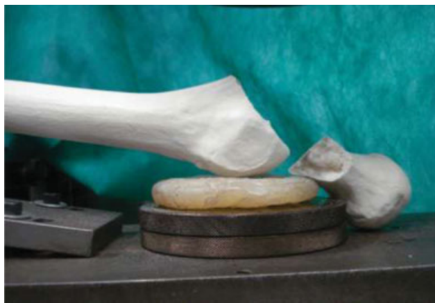
Fig. 4 Synthetic femur model with basal-cervical fracture.
